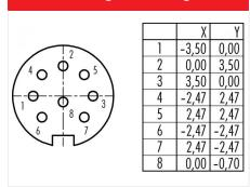
Contact arrangement (Plug-in side)
